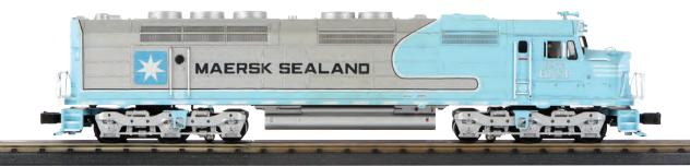
Designed in 1967 at the request of the Santa Fe, the FP45 was basically an SDP45 road switcher with a streamlined cab unit body. The "P" in FP45 indicated a passenger diesel with a steam generator for train heat. Having a sleeker, more aerodynamic look than a road switcher, the FP45 blended better with its passenger consists; the fully enclosed body also reduced wind resistance and allowed the crew to perform troubleshooting and minor maintenance on the road.
