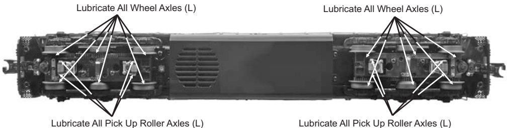
Figure 1: Lubrication Points on the Locomotive
