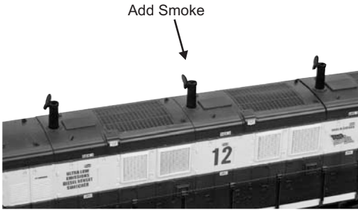
Figure 2: Adding Smoke Fluid
