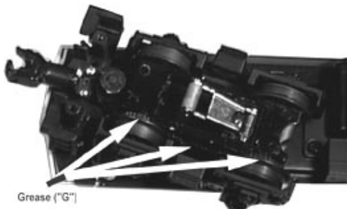
Figure 7: Lubricate The Tender Chassis Trucks
