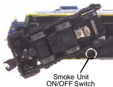
Figure 3. Smoke Unit ON/OFF Switch
