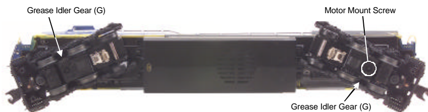
Figure 7. Locations of Greasing Points on the Locomotive
