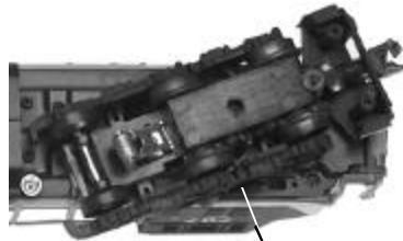
Smoke Unit Switch
