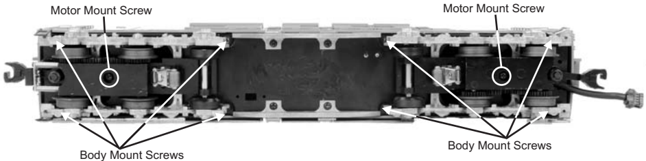
Figure 6b. B-Unit Body Removal Screw Locations
