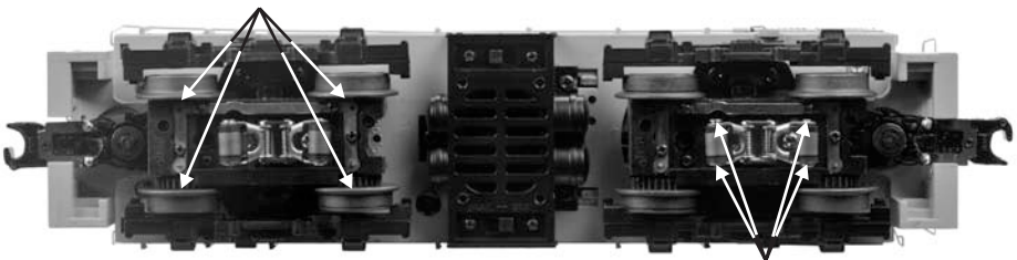
Figure 1: Lubrication Points on the Locomotive
