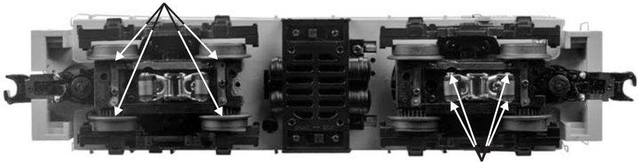
Figure 8: Lubrication Points on the Locomotive
