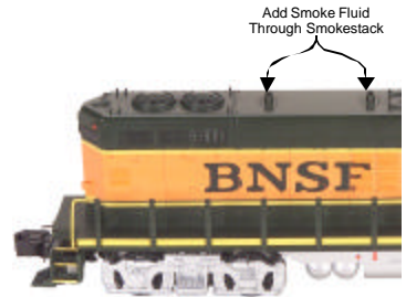
Figure 2. Add Smoke through the Smokestack
