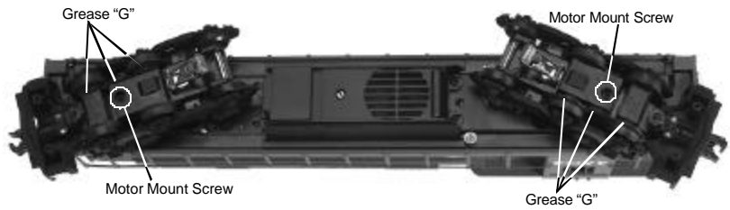
Figure 8: Greasing The Power Trucks
