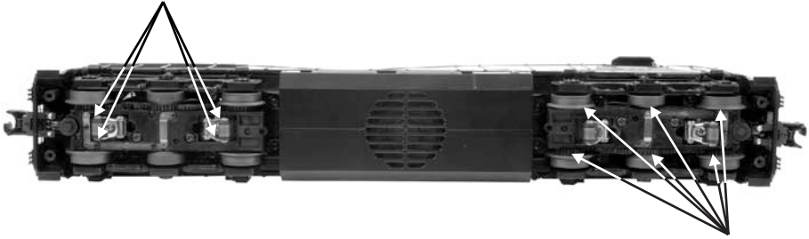
Lubricate All Wheel Axles (L)
