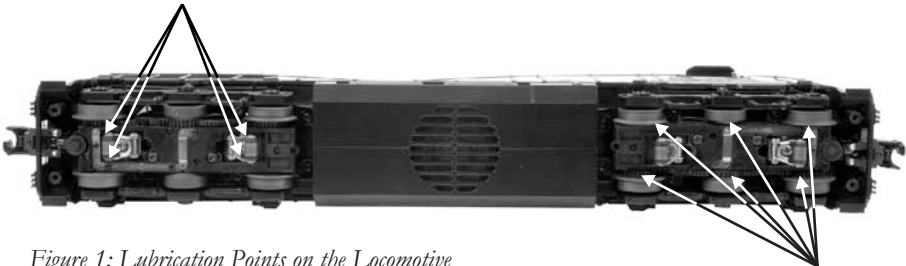
Lubricate All Wheel Axles (L)
