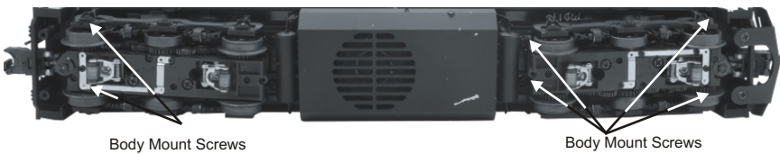
Body Removal Screw Locations
