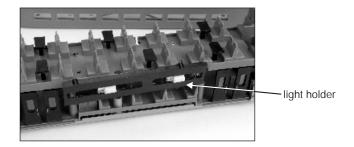
4. To remove the end bulbs pull the holder out of the guide and remove the bulb.
