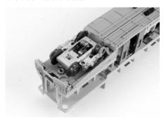
5. Line the spacer & Kadee Coupler up w/the holes in the undercarriage and screw them down.
