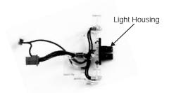
2. Pull the bulbs from the housing and remove the wires and 2-pin connector. Replace entire wire harness unit.
