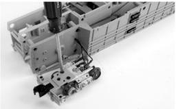
4. Attach the pilot to the bottom of the base. Then remove the coupler from the truck and reattach the truck to the base.
