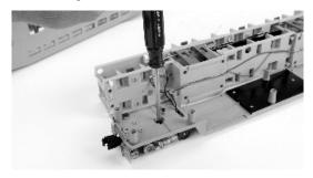
3. Remove the pilot from the truck by removing the 2 screws on top of the truck.
