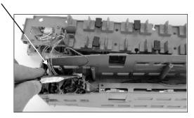
4. To replace the roof bulbs, grasp the base (not the bulb itself) firmly with a pair of needlenose pliers and pull gently. If you have difficulty reaching the bulbs, you may unscrew the roof light mount and remove it from the car for easier access.
