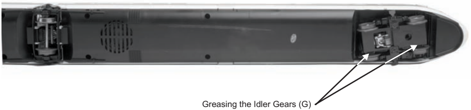
Figure 12: Greasing the Idler Gears
