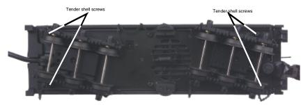
Figure 9. Screws to remove the tender shell
