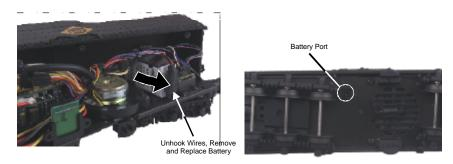
Figure 11. Replacing the Battery
