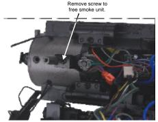
Figure 5a. Accessing the Smoke Unit
