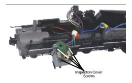
Figure 5b. Inspecting the Smoke Unit
