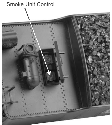
Figure: Smoke Unit Control
