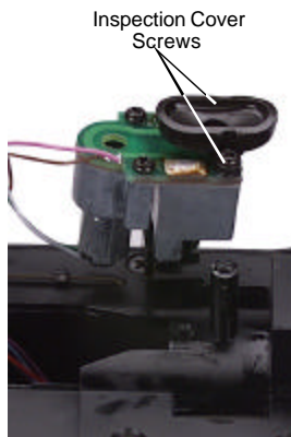
Figure 5. Inspecting the Smoke Unit
