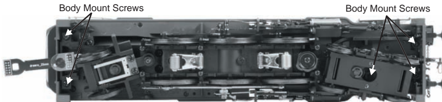
Figure 13: Removing the Body
