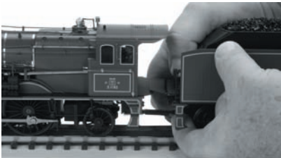
Figure 7: Connecting Locomotive to Tender
