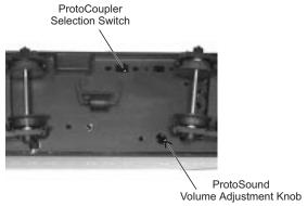
Figure 6: Adjusting The ProtoSound® Volume
