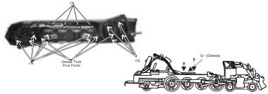
Figure 8: Lubricating The Locomotive Chassis
