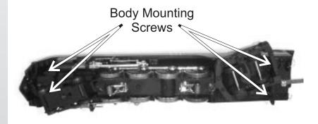
Figure 10: Removing The Body From The Chassis
