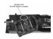
Figure 3: Smoke Unit Switch
