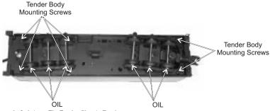
Figure 9: Lubricate The Tender Chassis Trucks
