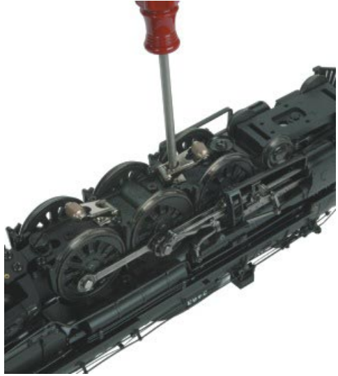
Figure 1: 3-Rail Pickups installed with a single Phillips Screw
