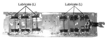
Figure 9: Lubricate The Tender Chassis Trucks
