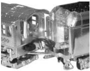
Figure 1: Pluging in in the tender harness
