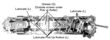
Figure 8: Lubricating The Locomotive Chassis
