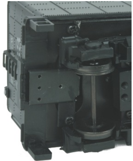
Figure 5: Pre-drilled Kadee® Coupler mounting holes
