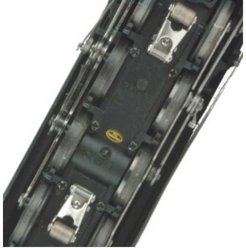
Figure 1: 3-Rail Pickups installed with a single Phillips Screw
