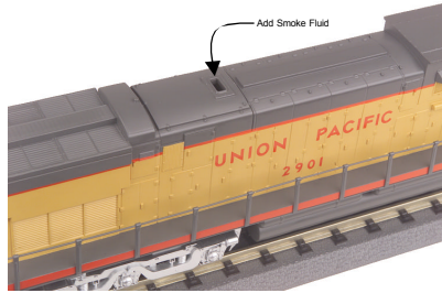
Figure 2: Adding Smoke Fluid
