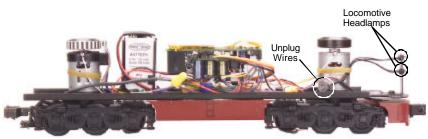
Figure 5. Location of the headlamp in the Engine.
