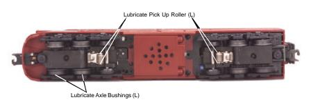
Figure 2. Lubrication Points on the Engine
