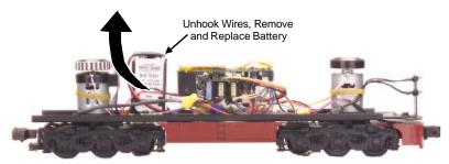
Figure 6. Removing and Replacing the Battery
