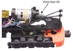
Figure 3a. Grease the Worm Gear
