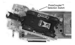
Figure 5: Proto-Coupler Selection Switch
