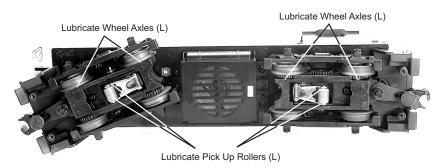
Figure 2. Lubrication Points on the Engine
