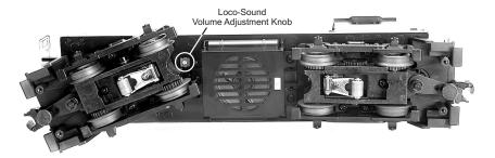
Figure 1. Location of the Loco-Sound Volume Adjustment Knob
