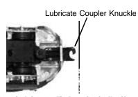
Figure 3: Lubricating The Proto-Coupler Knuckle
