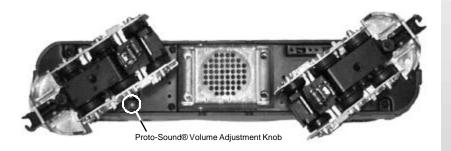
Figure 4: Adjusting The Proto-Sound® Volume
