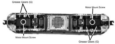
Figure 8: Greasing The Power Trucks
