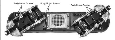
Figure 9: Removing the Body Mount Screws
