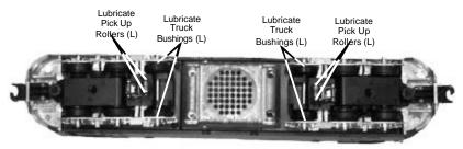
Figure 7: Lubricating The Truck
