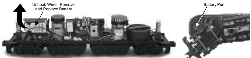
Figure 6. Unhook the Battery Leads, Remove the Battery and Replace with a New One.
