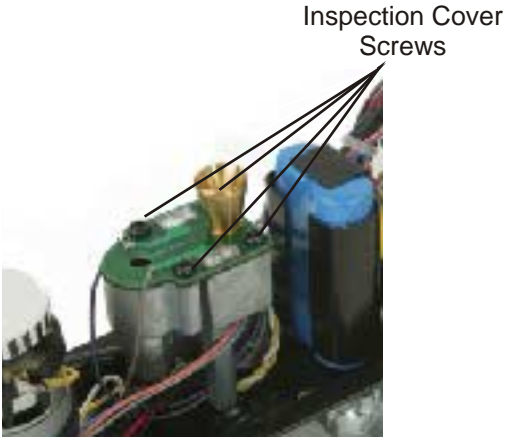
Figure 11. Inspecting the Smoke Unit Wick
