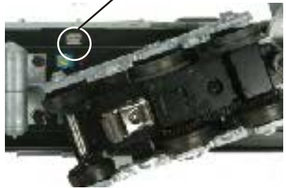
Figure 9. Battery Charger Port location.
