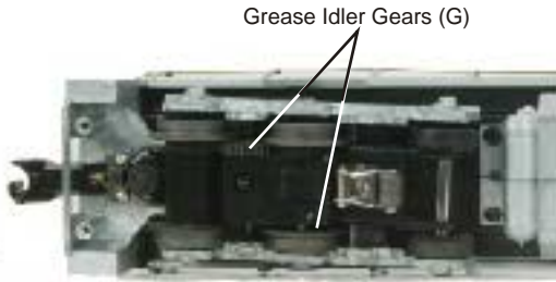
Figure 7. Greasing The Idler Gears
