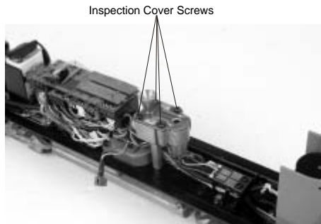
Figure 11 : Smoke Unit Inspection
