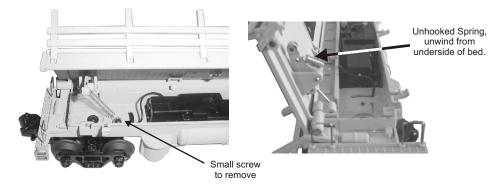
The spring that controls the dropping of the car side from underneath the bed may stretch too much to be effective if you repeatedly lift the bed too high off the base. To change the spring:
