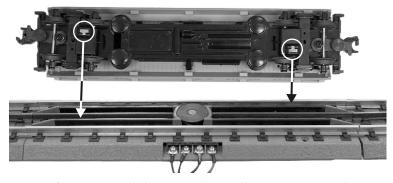
When you are ready to operate the log car, make sure the entire car is on the Uncoupling/Unloading Track Section (UTS\*), so that the car's slide shoe pick-ups are in contact with the fourth and fifth rails of the UTS. The recommended voltage for the dumping action is 10-14 volts.
