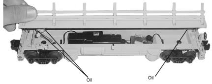
After several hours of use, you may notice a slowing of the dumping action. When this happens we recommend adding a light drop of oil to all the hinges. Be careful not to raise the bed too far or the springs will become stretched out.
