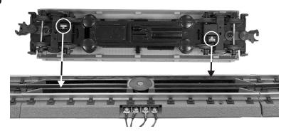
When you are ready to operate the dump car, make sure the entire car is on the Uncoupling/Unloading Track Section (UTS), so that the car's slide shoe pick-ups are in contact with the fourth and fifth rails of the UTS. The recommended voltage for the dumping action is 10-14 volts.
