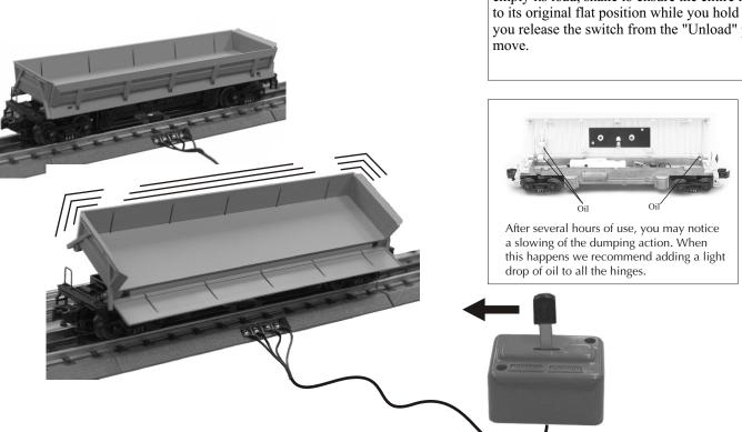
Hold the UTS switch in the "Unload" position. (Refer to your UTS instruction sheet for complete directions in its use.) The dump car will rise, empty its load, shake to ensure the entire load has been dumped, and return to its original flat position while you hold the switch in place. As soon as you release the switch from the "Unload" position, the car will cease to move.
