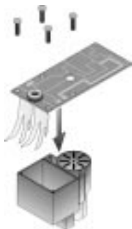
Figure 21: Opening the smoke unit for wick replacement.
