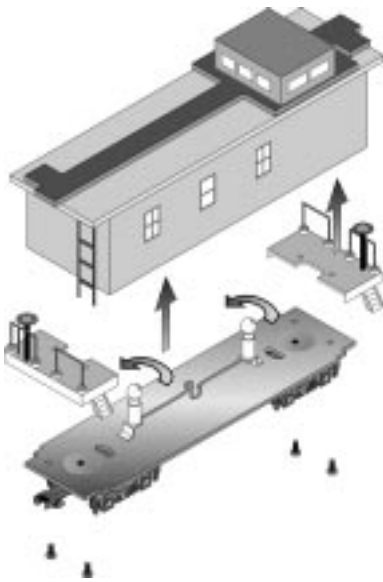
Figure 17: Removing the caboose body from its chassis.
