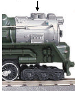
Figure 4. Add Smoke Fluid Through the Smoke Stack
