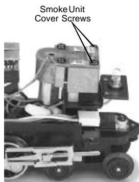
Figure 11. Inspection Cover Screws
