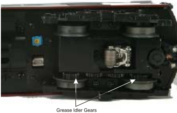
Figure 4. Greasing The Idler Gears
