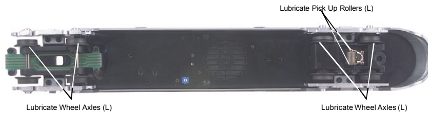
Figure 1. Lubrication Points on the Locomotive
