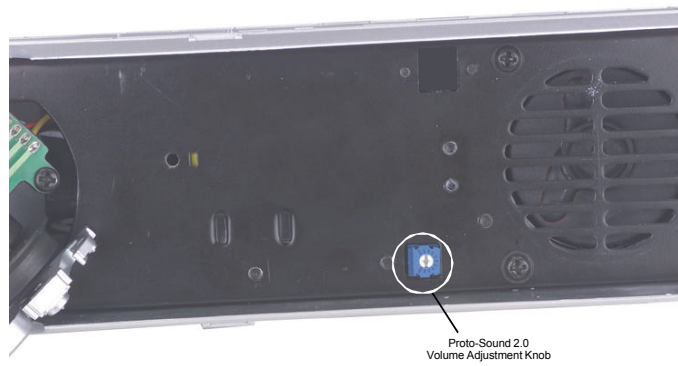
Figure 2: Manual Loco-Sound Volume Adjustment
