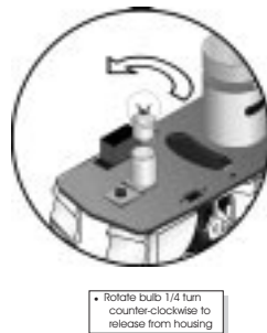
Figure 17: Removing the locomotive headlight bulb.
