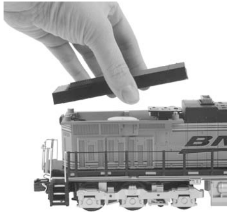
2. Remove Fan Cover to Access Smoke Unit and Volume Controls
