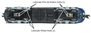
Figure 4: Lubrication Points
