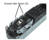
Figure 5: Greasing the Idler Gears
