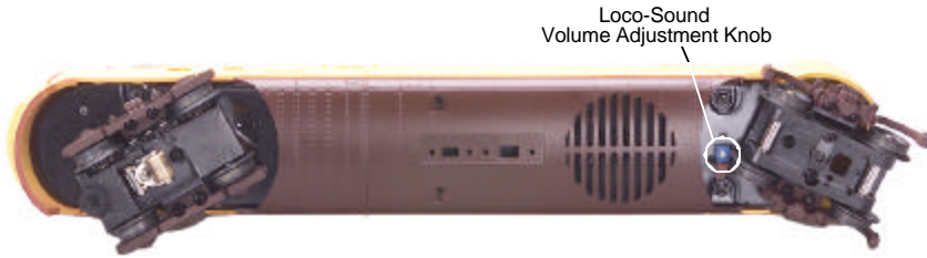
Figure 2. Location of the Loco-Sound Volume Adjustment Knob
