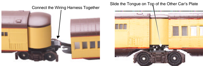
Figure 1. Connecting the Cars Together
