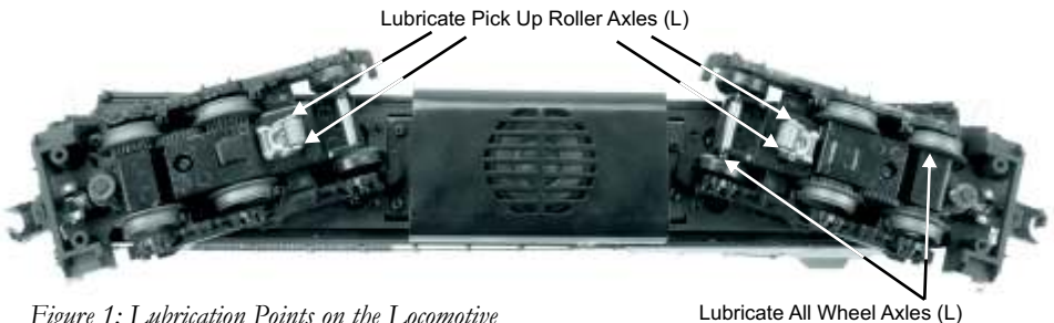
Figure 1: Lubrication Points on the Locomotive
