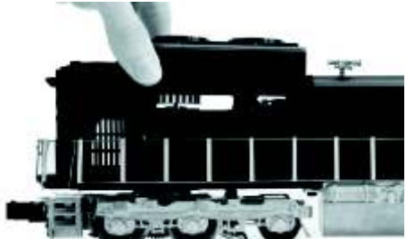
2. Remove Fan Cover to Access Smoke Unit and Volume Controls
