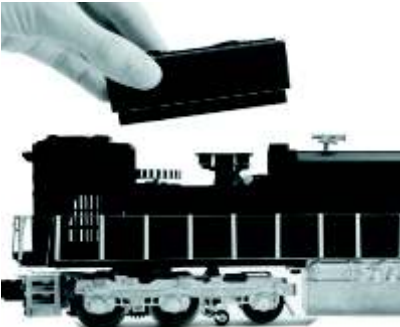
3. Fan Cover Removed
