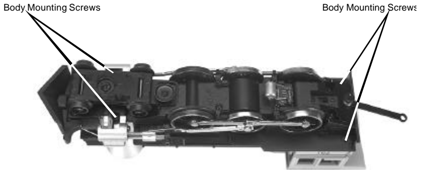
Figure 10: Removing The Boiler From The Chassis
