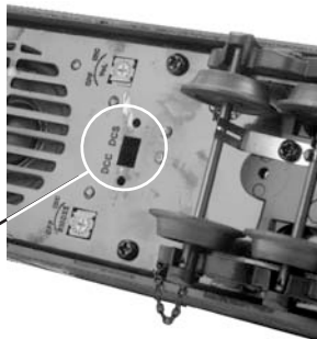
DCS/DCC Switch Location
