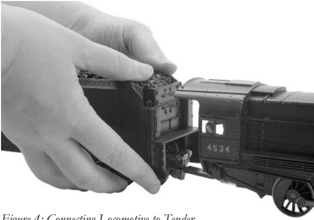
Figure 4: Connecting Locomotive to Tender
