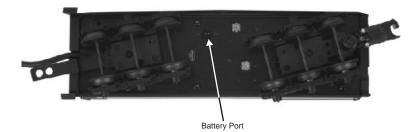
Figure 11. Battery Recharging Port
