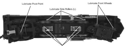
Lubricate Pick Up Rollers (L)
