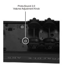
Figure 4. Manually Adjust The Volume
