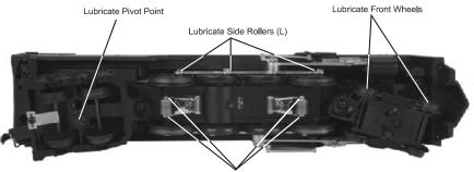
Lubricate Pick Up Rollers (L)
