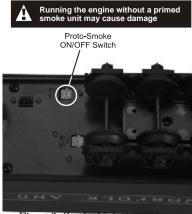
Figure 2. Smoke Unit Switch Location
