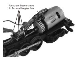
Figure 7. Motor Gearing Grease Plate Screws
