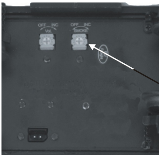
Figure 2: Smoke Unit Control
