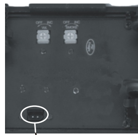
AC Battery Recharging Jack
