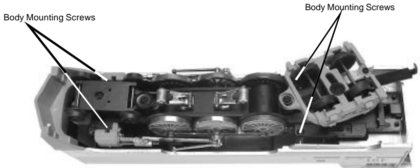
Figure 10: Removing The Boiler From The Chassis
