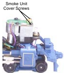
Figure 6. Smoke Unit Inspection Cover
