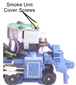
Figure 4. Smoke Unit Inspection Cover
