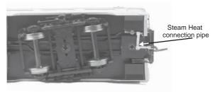
2. Remove the screw on the coupler pocket and remove the coupler from both ends of the car. (Be careful not to damage the coupler release bar.)
