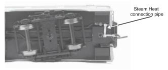
2. Then remove the screw on the coupler pocket and carefully move the coupler inward (Be careful not to damage the coupler release bar.)
