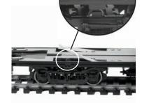
7) If you are still having problems with the car lighting up make sure the top of the contacts are bent up to make contact with the contact plates on the roof light board.
